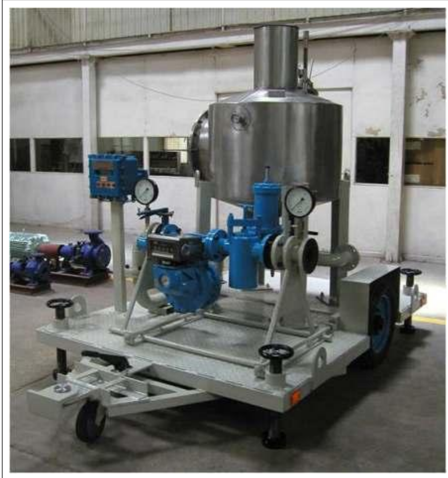
Custom Designed Mobile Skid Mounted Proving System
